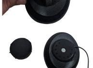
**C.3.** Install the speaker into the EarPad from the back.
