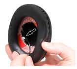
**A.6.** Using the Velcro, position and fix the speaker inside the NCS.
