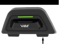
Hold the configuration button for 3 sec to access the configuration menu. You can then go to vehicle pairing by tapping the "up" button twice. Tap the center button to select "vehicle pairing". Then, on your vehicle display, go to Bluetooth settings and select your vibe product in the list of available devices.
